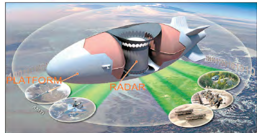
Long-term Surveillance: DARPA's Integrated Sensor Is Structure (ISIS) project is building a one-third-scale prototype of an unmanned, radar-carrying blimp that can stay aloft for a decade.
